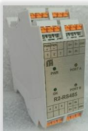
Modular repeater **R2-RS485** type is designed to increase the length of the communication line RS-485 by repeating the electrical signal, as well as to increase the range of Modbus devices.
