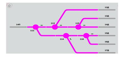
Using KS-01 or a switch on the track box the command is sent to move the turn-out to the "plus" or "minus" position. The position indication of the point machine is shown on the KS-01 console and by the point indicator, which is installed in front of the turn-out and indicates the direction.
