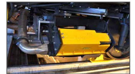
On permanent installations the LTM Protect fan system keeps the lenses clean
